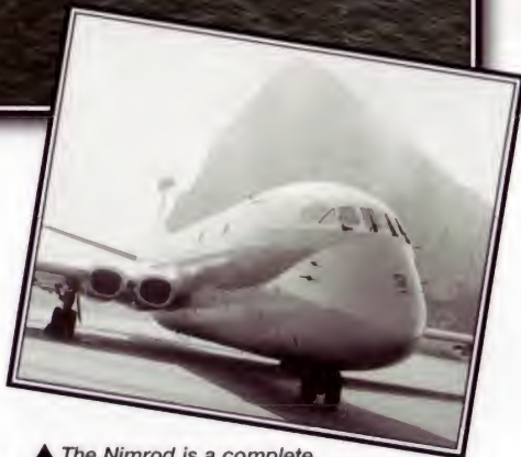
▲ The Nimrod is a complete anti-submarine and anti-ship battle station. Its unique four-jet configuration allows the aircraft to chase a contact faster than any other maritime aircraft.
